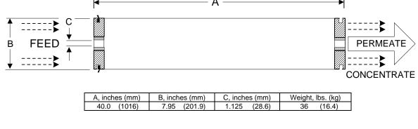
Notice: Permeate flow for individual elements may vary + or - 15 percent. All membrane elements are supplied with a brine seal, interconnector, and o-rings. Elements are vacuum sealed in a polyethylene bag containing less than 1.0% sodium meta-bisulfite solution, and then packaged in a cardboard box.
