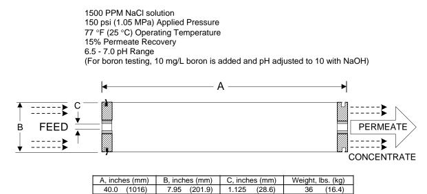
Notice: Permeate flow for individual elements may vary + or - 15 percent. All membrane elements are supplied with a brine seal, interconnector, and o-rings. Elements are enclosed in a sealed polyethylene bag containing less than 1.0% sodium meta-bisulfite solution, and then packaged in a cardboard box.
