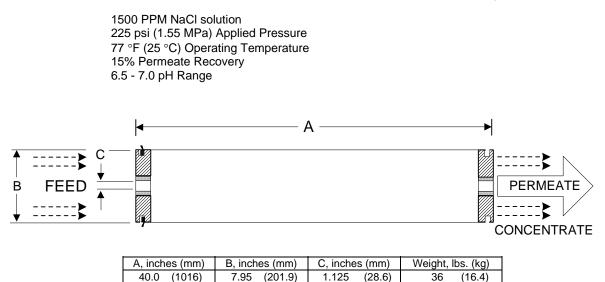
Notice: Permeate flow for individual elements may vary + or - 15 percent. All membrane elements are supplied with a brine seal, interconnector, and o-rings. Elements are vacuum sealed in a polyethylene bag containing less than 1.0% sodium meta-bisulfite solution, and then packaged in a cardboard box.
